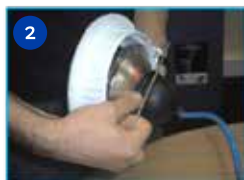
2. Remove spring retainer from terminal cap
