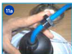
11. Ensure o-ring is in place and gland nut is tightened
