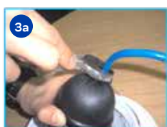
3. Remove the terminal cap from the globe by loosening the nut
