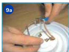
9. Place terminal flags on lugs of LED globe
