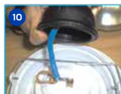
10. Replace terminal cap with o-ring in place
